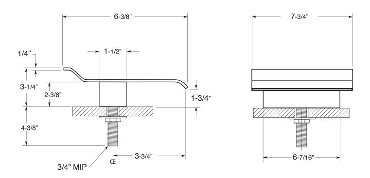
NOTE: Spouts install through 1-1/4" Diameter Holes.
