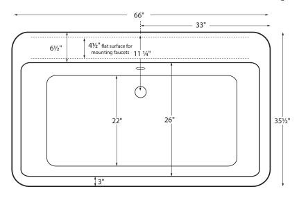
Features a 4.5" wide flat deck surface on the drain side for mounting faucetry.
