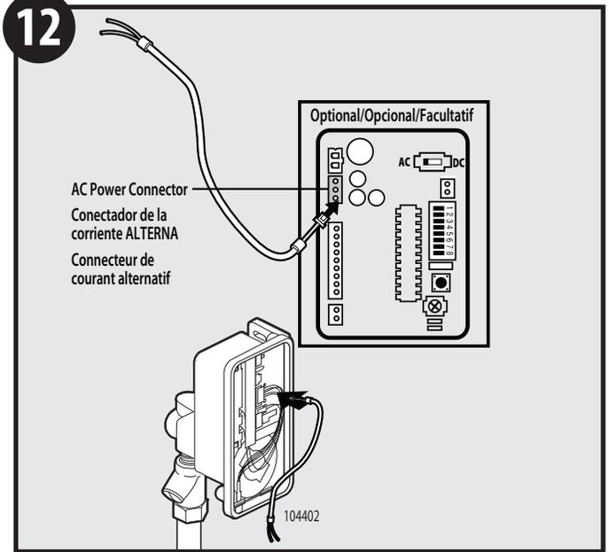
Connect the 3-pin connector of the 104402 wire lead to the 3-pin connector housing on the printed circuit board.
