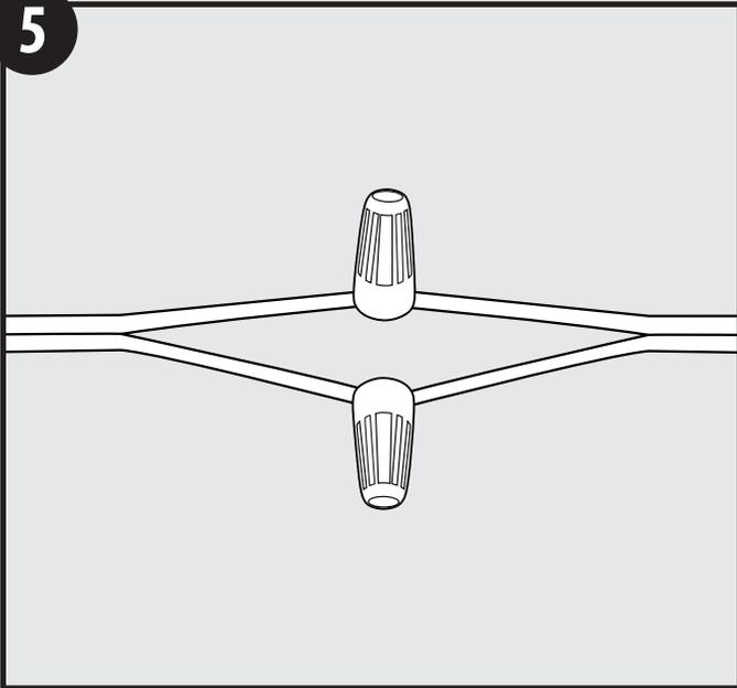
Using wire nuts, connect each strand of the 18 gauge wire to one of the two output lead wires of the transformer, as shown. Ensure that the strand of the 18 gauge wire extension that is connected to the positive (+) (non-ribbed) output lead wire of the transformer (wire with white lettering/printing on it) is distinguishable as the positive (+) strand.
