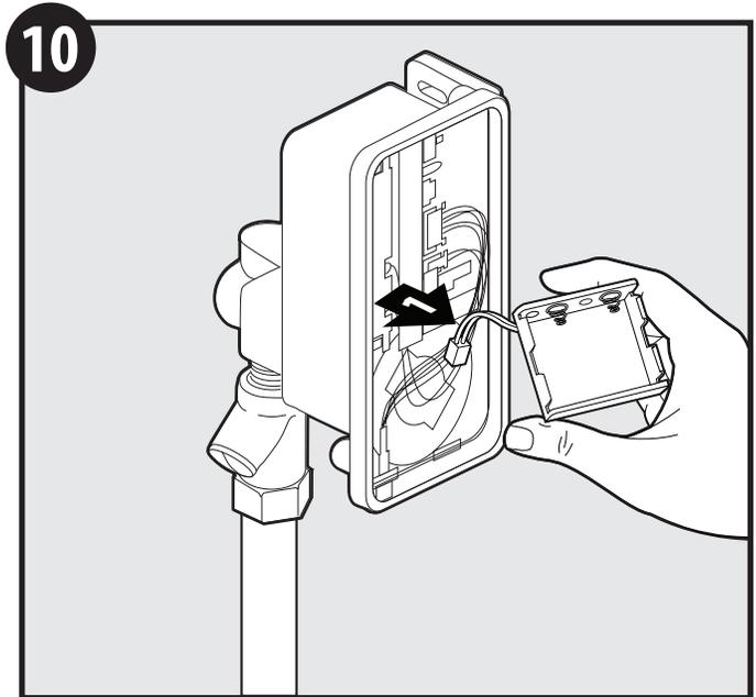
Remove the battery holder's cable connector from the printed circuit board, and place battery holder and batteries aside. They are no longer required.
