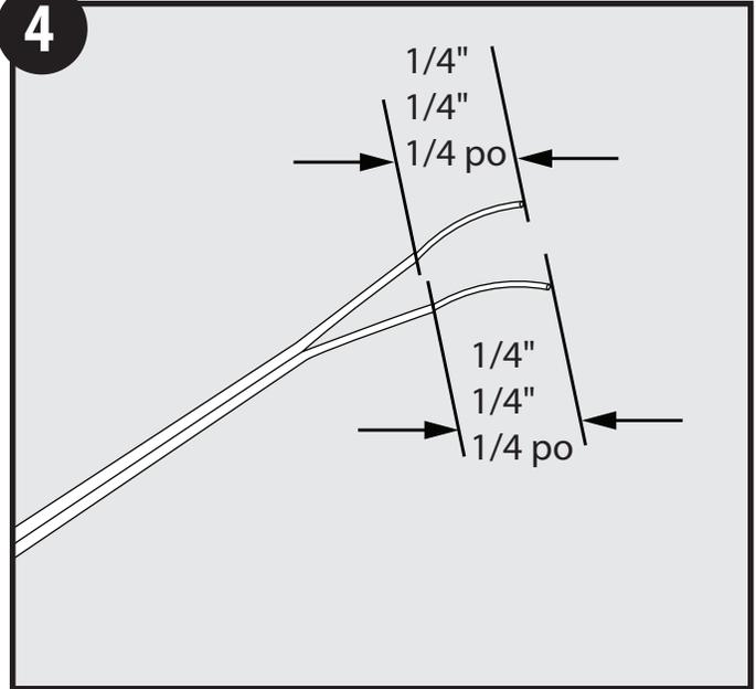
Measure and cut a dual strand 18 gauge wire to the length required to extend the transformer's output lead wire to the faucet or flush valve furthest from the mounting location of the transformer. Strip about 1/4" of the insulation off both ends of each strand of the 18 gauge wire.
