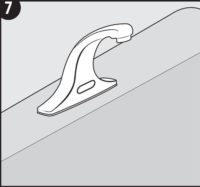
If not already installed, install each of the faucets or flush valves to be powered by the transformer per their installation instructions. Once installed, ensure that the water supply(s) to the faucets or flush valves is turned off.
