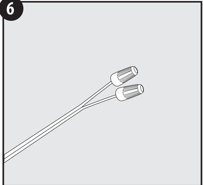
Place wire nuts over each exposed end of the transformer's output lead wire, as shown.
