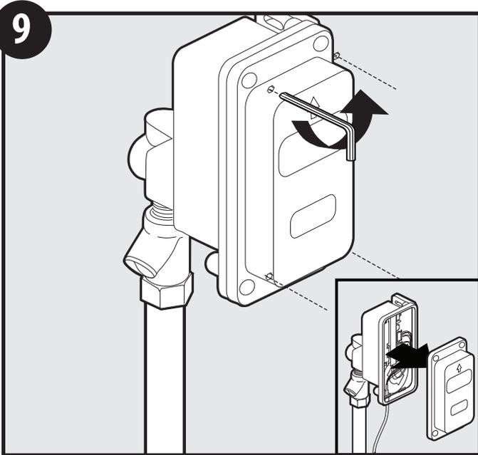
Open the electronics box underneath the sink deck for the first faucet to be connected to the 104401 transformer, by removing the four (4) socket head cap screws.
