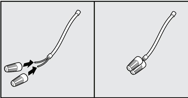
• Do not touch bare ends of transformer output lead wires together when transformer input lead is plugged into electrical wall outlet; avoid contact by using electrical wire nuts as shown during installation.
