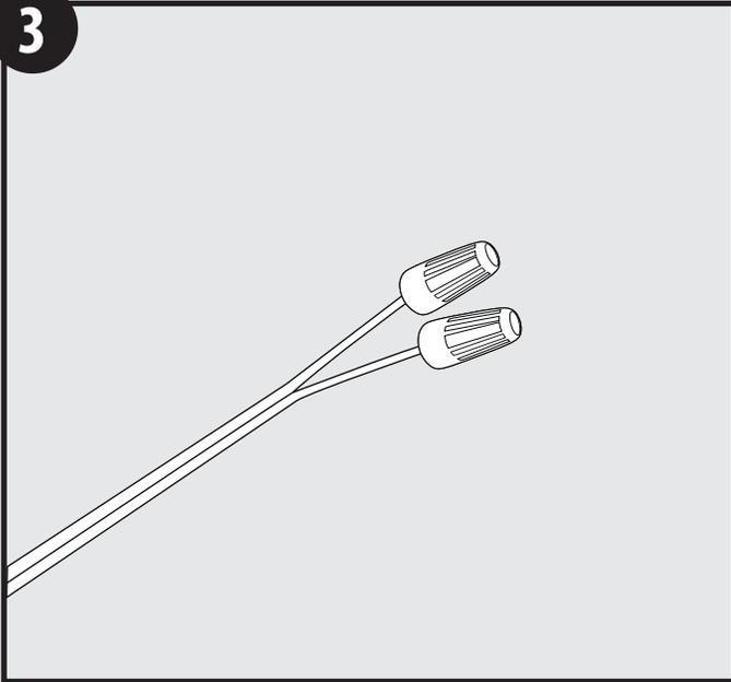
Determine if an extension to the transformer's output lead is required to reach the faucet or flush valve furthest from the mounting location of the transformer. If so, proceed to step 4. If not, place wire nuts over each exposed end of the transformer's output lead wire, as shown and proceed to step 7.
