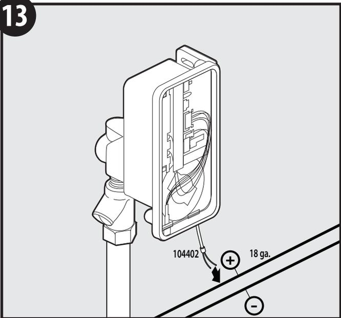
Replace the printed circuit board in the electronics box, allowing the wires of the 104402 wire lead to exit the electronics box thru one of the wire openings at its base.
