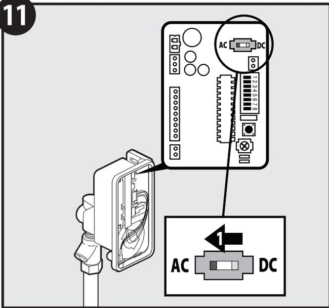
Set the AC/DC switch on the printed circuit board to the AC setting.
