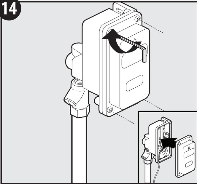
Replace the cover of the electronics box, and secure it by tightening the four socket head cap screws.
