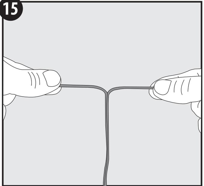
Carefully split the positive (+) (non-ribbed) and negative (-) (ribbed) strands of the transformer's output lead wire (or the positive (+) and negative (-) strands of its dual strand 18 gauge extension wire), so as not to damage, or otherwise compromise the wire insulation, as shown, at a location where the wire leads from the faucet or flush valve can be tee connected into the transformer's output lead wire.
