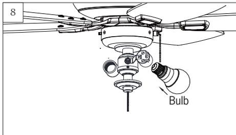
Install 2 x 9-watt medium base enclosed type of LED lamps.
