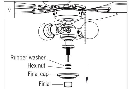
Remove finial, final cap, hex nut and rubber washer from light fixture. Keep the parts.
