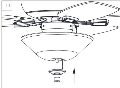
Align hole in center of final cap with thread rod, allowing pull chains to come through appropriate holes in the final cap, and push up. Thread center pull chain through hole in finial and secure glass to light fixture by tightening the finial. **DO NOT OVER TIGHTEN** the finial as glass may crack or break.
