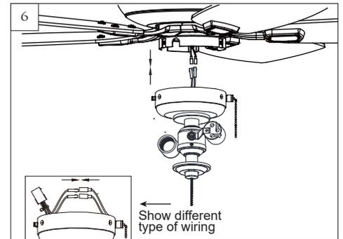
Connect white wire from light fixture with white wire from fan and then connect black (or blue) wire from light fixture with blue (or black) wire from fan.
