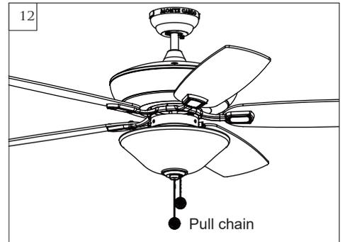
Install fan and light kit pull chains to preassembled pull chains on fan. Pull chains provided.
