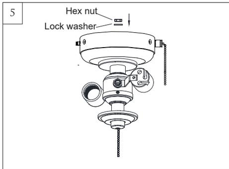
Place lock washer and hex nut provided over lead wires from light fixture and tighten securely with the thread rod of light fixture.
