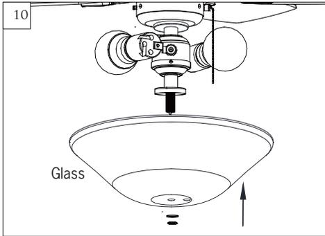
Raise glass in order to guide pull chains through appropriate holes in glass, aligning threaded rod on light fixture with hole in middle of the glass and push up gently allowing threaded rod to come through hole. (**Note:** Be sure pull chain for fan operation does not rub against bulb during operation).
