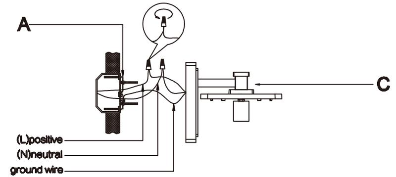
2. Caulk around backplate where fixture meets the wall leave a hole at the bottom to allow water to escape.
