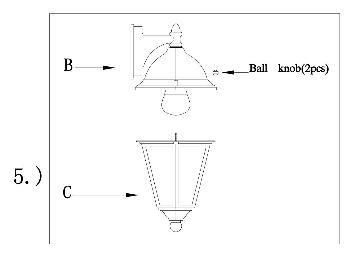
Step.5: Attach cage(C) to fixture, using ball knobs.
