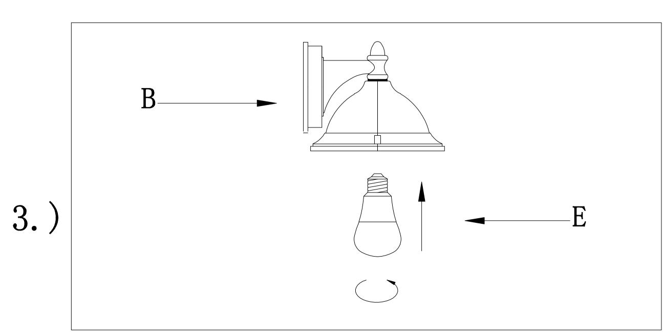
Step.3: Install E26 LED bulb(E)
