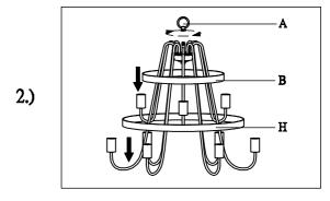
Attach top loop (A) and run ring (B) and (H) over the top and bottom arms. Open the arms and allow for the ring to sit evenly over them.
