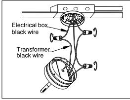
Step 6.Tuck the wire nut connections into the electrical junction box. Slide the transformer housing up until the holes line up to the back plate,make sure all wires are tucked in. secure it in place with the 3 screws previously removed. Note: MAKE SURE THAT THE STAND OFF IS IN ALIGNMENT WITH THE RAIL.
