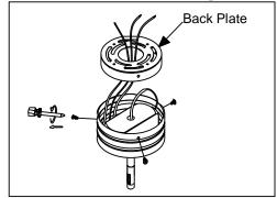
Step 3.Line up the back plate with the two screw holes from the junction box and secure the two screws supplied with the junction box.
