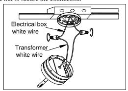
Step 5.Connect the black (hot) wire from the transformer to the black wire from the junction box use a wire nut to secure the connection.
