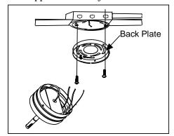
Step 4.Connect the bare (ground) wire for the transformer to the bare or green ground wire from the junction box use a wire nut to secure the connection.
