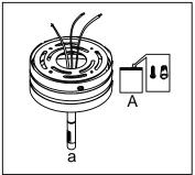
Step 2.Remove and set aside the 3 screws from the transformer to release the back plate.
