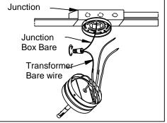
Step 4. Connect the white (neutral) wire from the transformer to the white wire from the junction box . use a wire nut to secure the connection.
