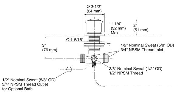
Can be installed in a wall-mount application to the same roughing-in dimensions.
