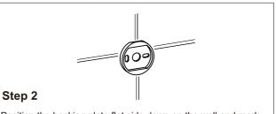
Position the backing plate flat side down on the wall and mark holes with pencil.
