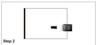
Use an appropriate amount of UV shadowless adhesive to the surface of the glass to be adhered, then close it with the solid backing to expel possible bubbles.
