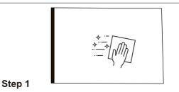
Ensure that the glass is clean, dry, free of grease, and flat. (The grease, moisture, impurities, and flatness on the surface will directly affect the quality.)
