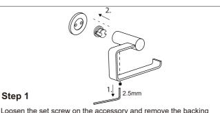
Loosen the set screw on the accessory and remove the backing plate. Position the accessory against the wall and mark outline with pencil.
