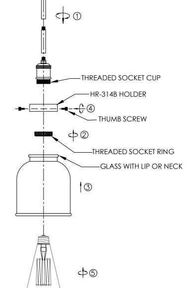
OR NECK THE HR-314B HOLDER IS NEEDED TO ATTACH THE GLASS
