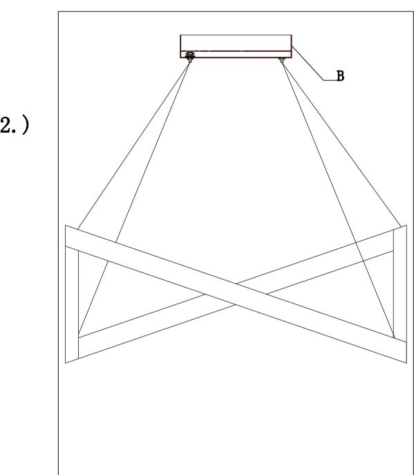
Step.2: Adjust wire length to desired mounting height, and tighten strain relief screws to secure. Wire fixture to wires in outlet box. Install fixture to bracket and tighten screws at the ends of the canopy to
