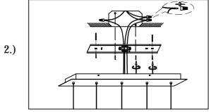
Step.2: Wire fixture to wires in outlet box. Green wire is for Ground.
