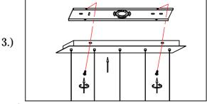
**Step.3:** Tighten screws on the sides of the canopy (C) to secure the fixture.
