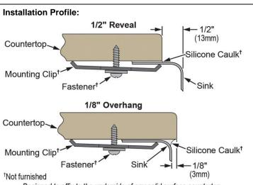
Designed to affix to the underside of any solid surface countertop.
