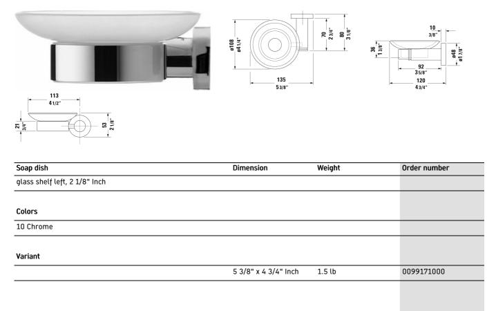
All drawings contain the necessary measurements which are subject to standard tolerances. They are stated in inch & mm and are nonbinding. Exact measurements, in particular for customized installation scenarios, can only be taken from the finished ceramic piece.
