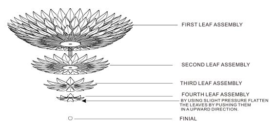
NOTICE: FOR REPLACING THE BULB, PLEASE UNSCREW THE LEAF ASSEMBLY AS SHOWN ABOVE
