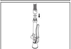
(6) Make sure hose washer is inside 20" hose connection end and tighten spray valve to 20" hose with wrench.
