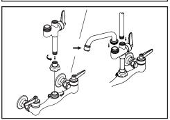
(3b) Attach body adapter to inlet of add-on faucet with Allen wrench. Apply Teflon tape to thread end of overhead swivel unit then thread overhead swivel unit to add-on faucet, attach add-on faucet to faucet body by tightening body adapter with wrench then attach spout to add-on faucet, go to step (5).
