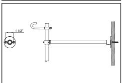
(5) Install 12" adjustable wall bracket and cut the excess support arm to fit in proper distance from wall to overhead swivel unit. Attach finger hook & screw, adjust to proper position.
