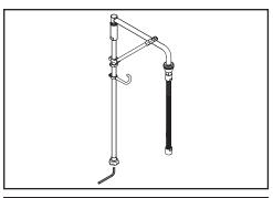
(3a) If there is no add-on faucet, please go to step (4). Remove body adapter from overhead swivel unit with Allen wrench supplied with add-on faucet.
