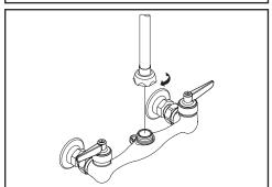
(4) Attach overhead swivel pre-rinse assembly to faucet body by tightening body adapter with wrench.
