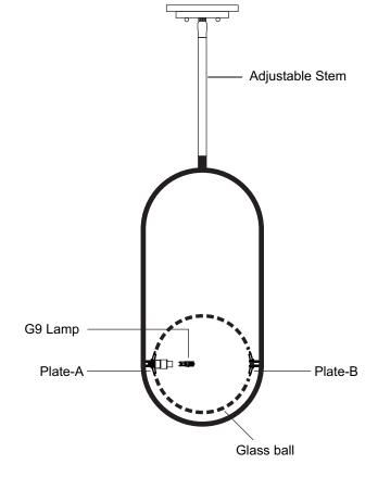
9. Install the glass ball to the fixture by securing it with plates A & B. (See Figure-03)
